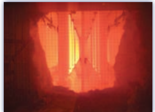
Glass is fused to steel at 1,500°F (816°C) in a state-of-the-art furnace.
